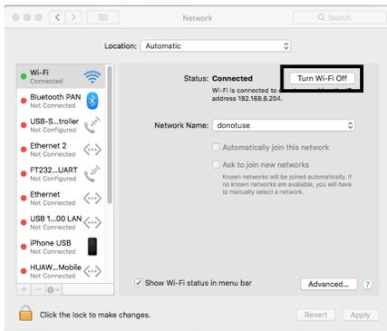
Select Ethernet from the left menu and in case input fields are grayed out, unlock settings by clicking on the Lock in the bottom left corner.
