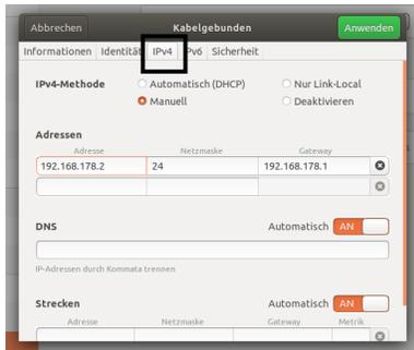
Now you will need to deactivate and reactivate the network interface to correctly apply the settings. Do so by turning the connection from On to Off. Wait two seconds and turn the connection back On again.
